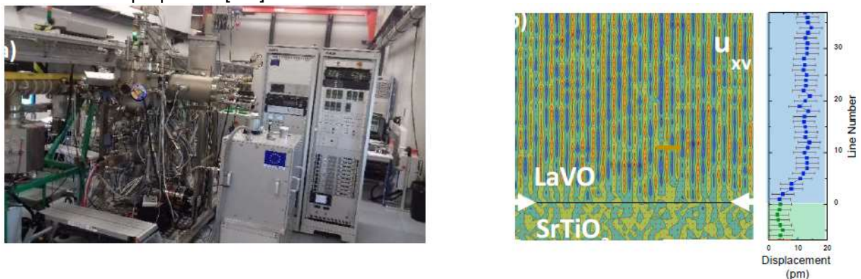
Fig. 1: (a) Picture of the IJL ozone-MBE connected to the Dapm equipment at IJL (b) Local displacement of RE atoms extracted from HRTEM observation of a LaVO_3 epitaxial film.
