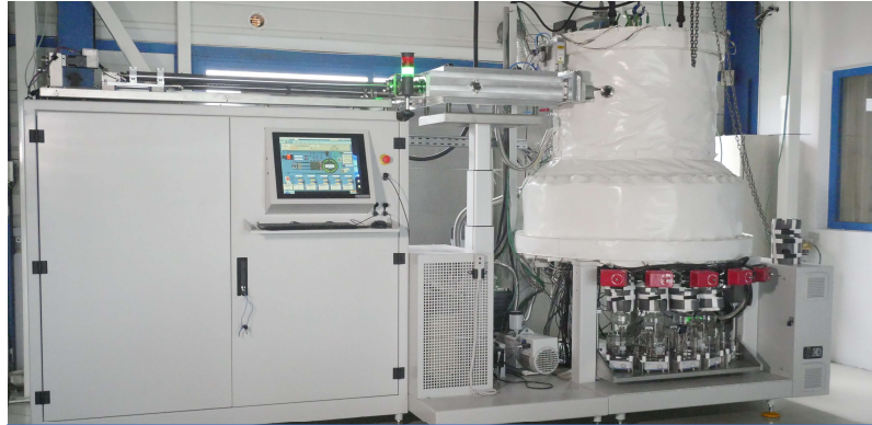
SINGLE WAFER SYBILLA-450 MM MERGING CVD AND MBE ASSETS
