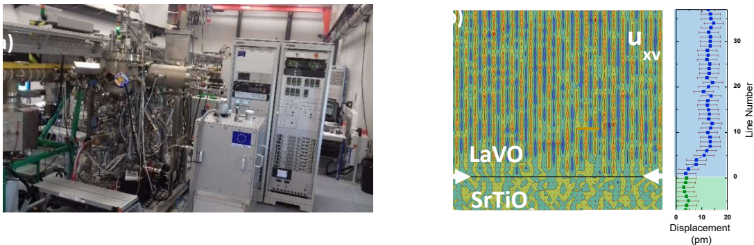
Fig. 1: (a) Picture of the IJL ozone-MBE connected to the Daum equipment at IJL (b) Local displacement of RE atoms extracted from HRTEM observation of a LaVO_3 epitaxial film.
